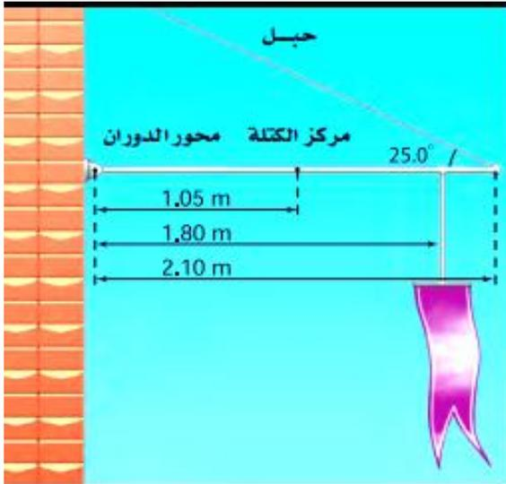
$$F_1 r_1 \sin \theta = F_2 r_2 + F_3 r_3$$
