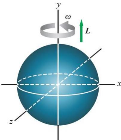
$$m = 5.0 \text{ kg}, r = 10.0 \times 10^{-2} \text{ m}, \omega = 20 \text{ rad/s}, I = \frac{2}{5} mr^2$$
