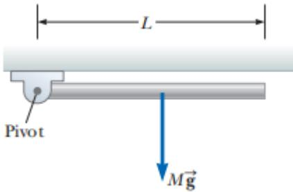
$$\begin{aligned}\sum \tau &= I \alpha \\ \alpha &= \frac{\tau}{I} = \frac{Mg \frac{L}{2}}{\frac{1}{3} M L^2} = \frac{3g}{2L} \\ &= \frac{3(10)}{2(1)} = 15 \text{ rad/ s}^2\end{aligned}$$
